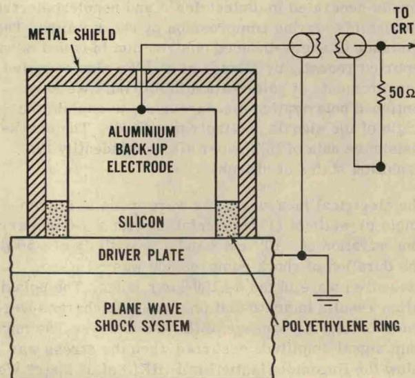
FIG. 1. Experimental arrangement for observing shock-induced electrical signals.
